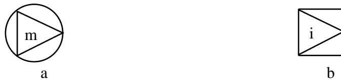
Figure 1. Material type port (a) and information type port (b). The triangle shows the direction – the edge is pointed to the exterior ( out port) or interior ( in port) of the entity that contains it. The label is written inside.
