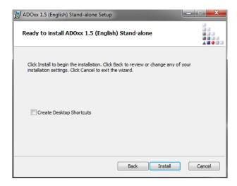
Start the installation by clicking on "Install". In case you want to create desktop icons during the installation, select the checkbox.
