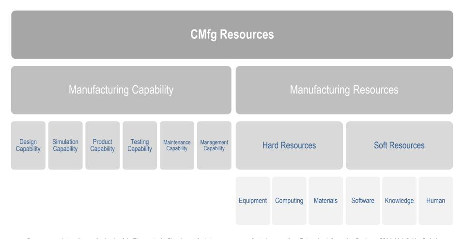
Source: own elaboration on the basis of: L. Zhang et. al., Cloud manufacturing: a new manufacturing paradigm, Enterprise Information Systems, 2014, Vol. 8, No. 2, 1–1
